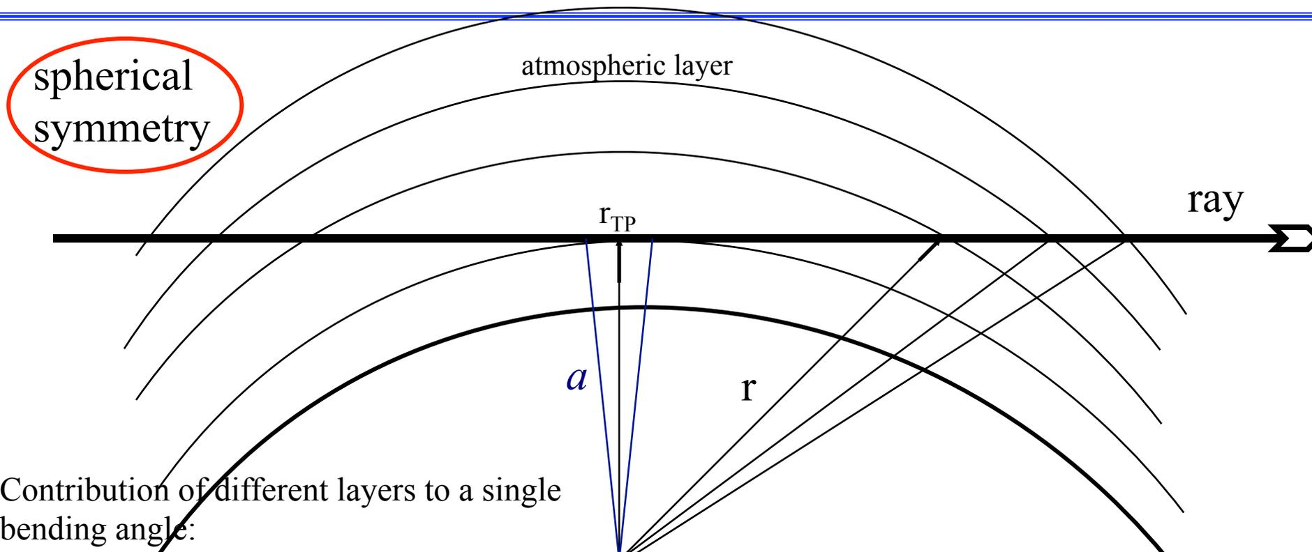
Contribution of different layers to a single bending angle:
